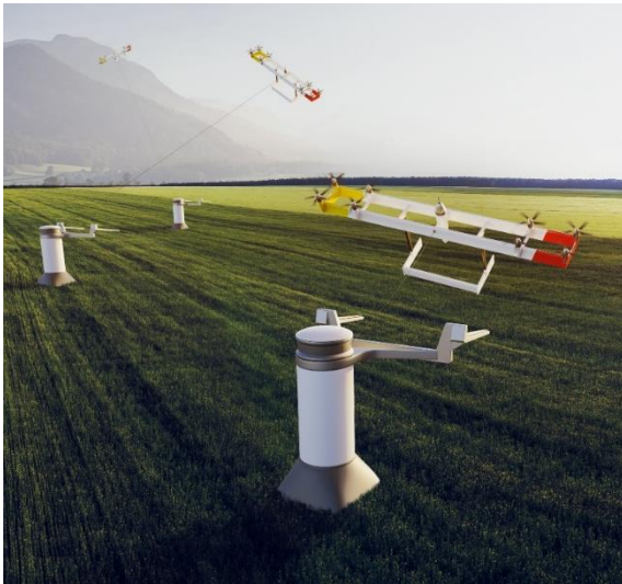
Left: 3D rendering of the rigid drag power kite developed by Kitekraft. Source KiteKraft [1].
