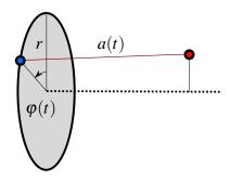
However, if we add a number of similar sources equally spaced around this circle, it is not fully clear how the single sound waves of each source superimpose and whether this interaction leads to a beating sound experience at the receiver position (red dot). Therefore, this circumstance must be analyzed and understood in more detail. The results would close a gap between the Doppler effect and the beating effect.
