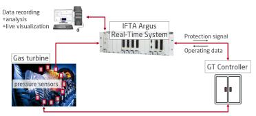
Control of an industrial gas turbine using online monitoring.
