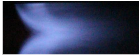
Figure 1: Lean combustion zone in the RQL combustion test rig
