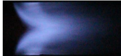
Figure 1: Lean combustion zone in the RQL combustion test rig
