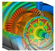
thermal management. Using a predefined motor geometry, various influential parameters – such as cooling methods and magnet configurations – will be evaluated through simulation-based approaches.
