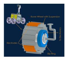
defined system to apply dust to the slip ring shall be built as a part of the setup to test different sealing options of the prototype slip ring.
