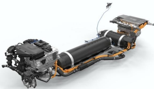
Figure 1: Drive system of the BMW iX5 Hydrogen [bmwgroup.com]
