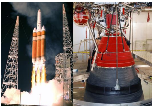
Figure 1: The launch of Delta IV Heavy (left), CNE of the Delta IV upper stage (right) [Wikipedia].
