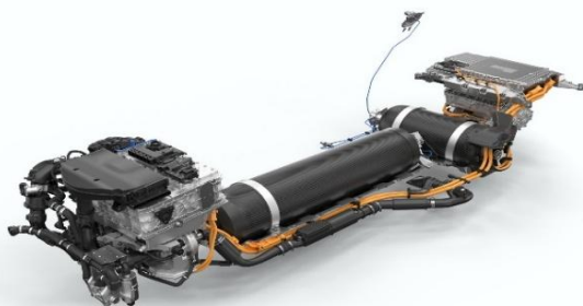
Figure 1: Drive system of the BMW iX5 Hydrogen [bmwgroup.com]
