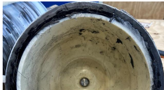
Figure 2: Cross section of Thermoplastic Type-4 PV
