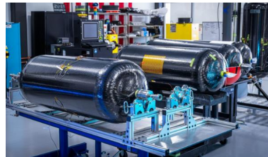
Figure 2: COPVs for spacecrafts [dawn aerospace.com]
