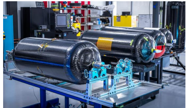
Figure 2: COPVs for spacecrafts [dawn aerospace.com]
