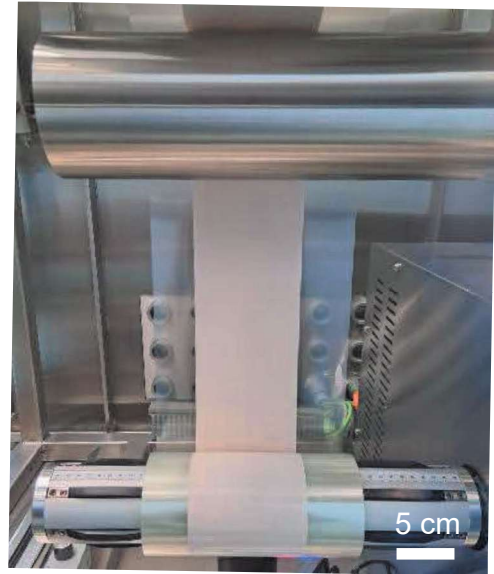
Figure 1: Roll-to-roll coated separator for sulfide-based solid-state batteries
