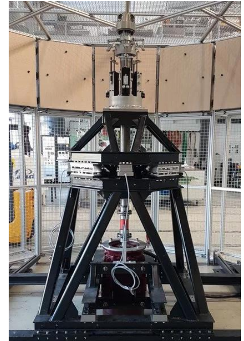
Fig 1: The MERIT Test rig, without blades attached
