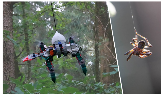
Tethered suspended drone stabilizing on an oscillating branch.
