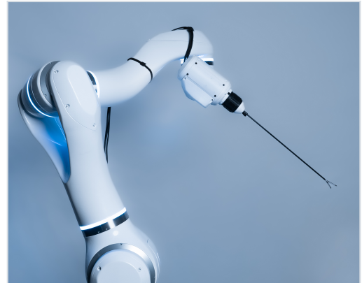
Surgical robotic platform developed for our ASSIST project, utilizing Karl Storz Clickline Instruments.
