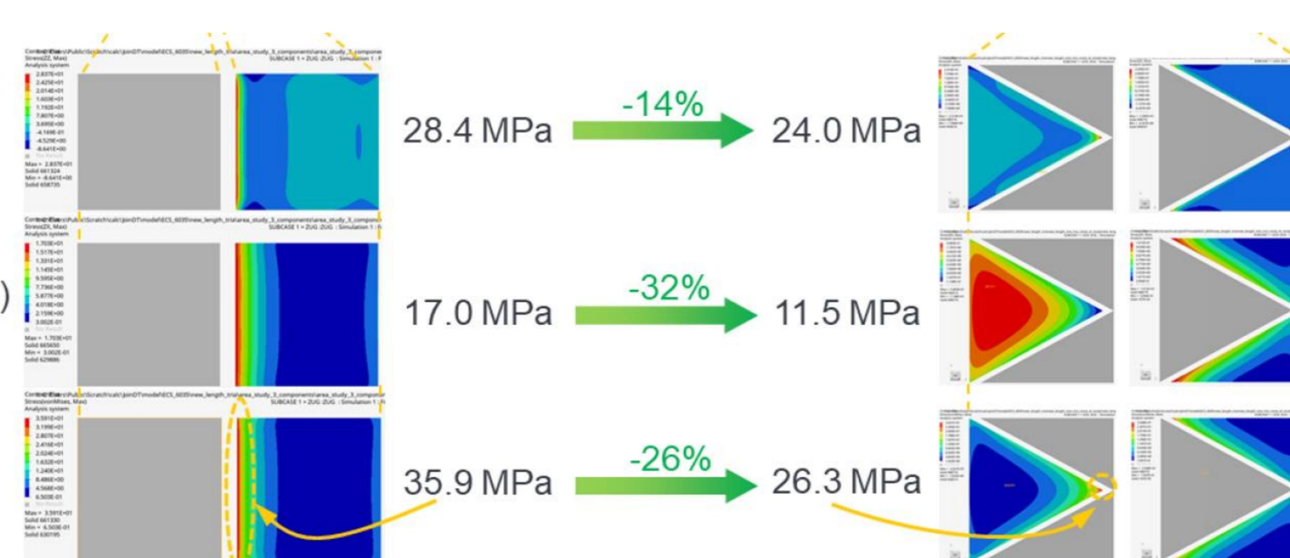
Figure: Stress comparison between conventional and damage-tolerant bonds.
