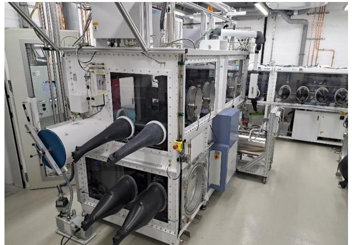
Pilot scale production line for solid state batteries at the iwb
