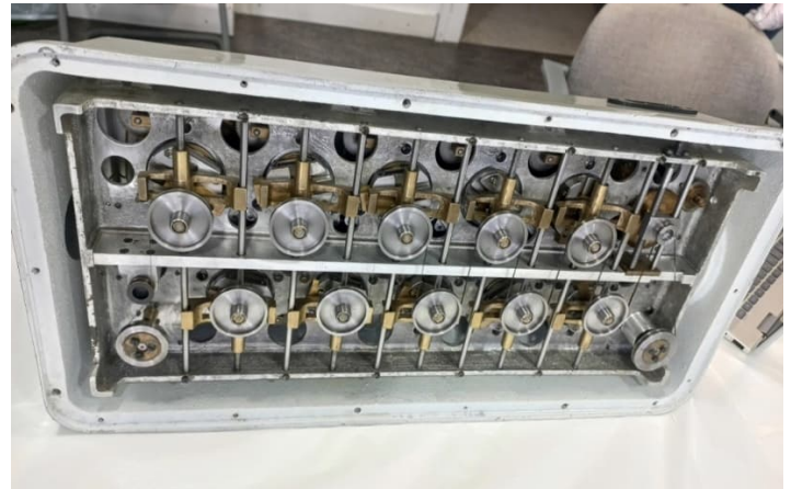
Figure 2: Parts of the internal structure of the tide calculator under examination. Image credit: Deutsches Museum.
