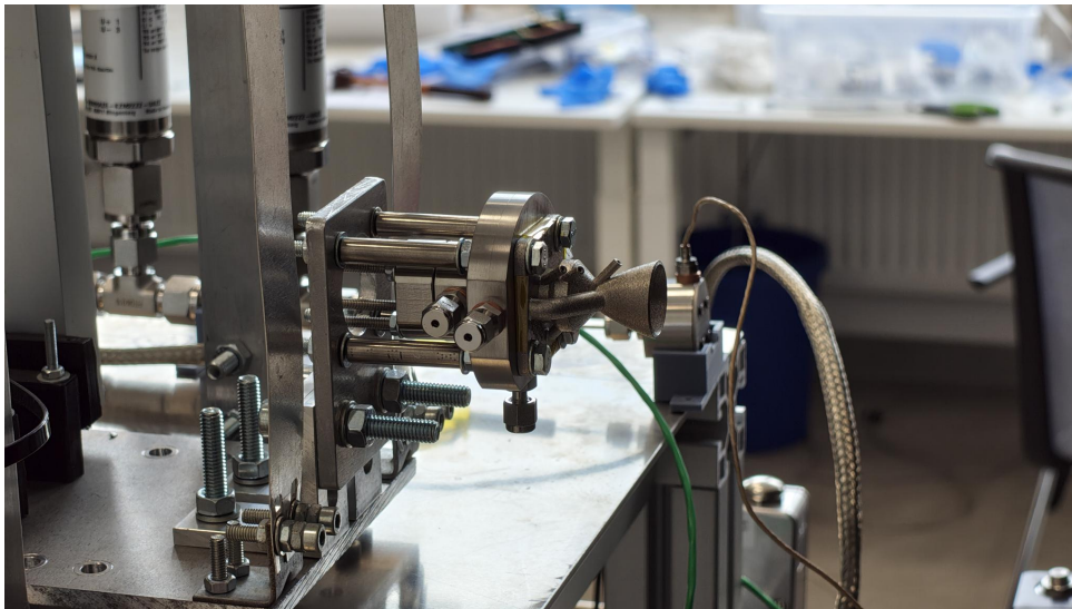
Figure 1: Ice2Thrust hot-gas thruster and thrust balance currently in use
