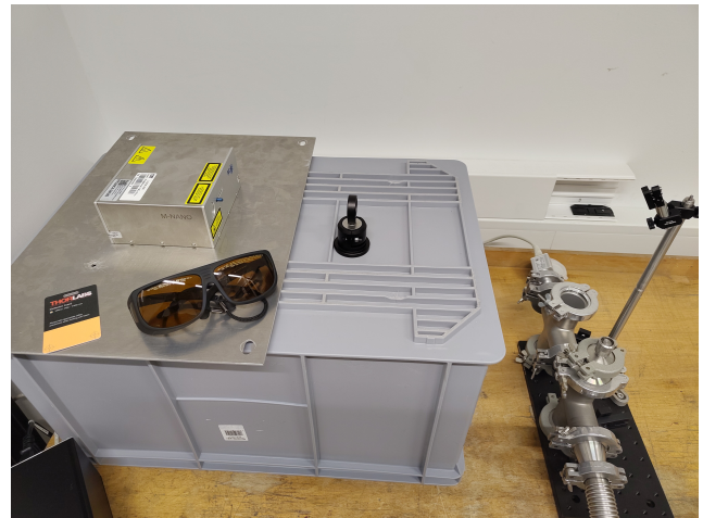
Figure 1: Current laser and vacuum chamber setup.
