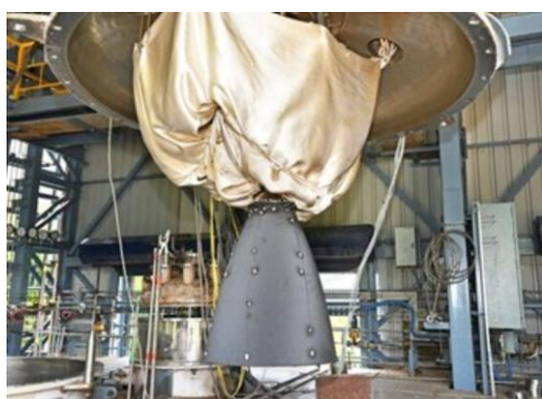
Figure 1: C/C composite nozzle attached to PS4 engine of ISRO's workhorse launcher [ISRO].
