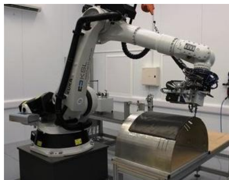
Figure 2: Tufting of CF components with complex geometries for aerospace applications [Dell'Anno et al. 2015].
