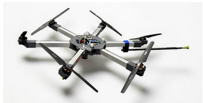
Figure 1: Fully actuated aerial manipulator platform with an end-effector, used for indoor control, state estimation, and interaction-force estimation methods.
